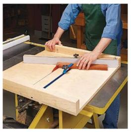
The illustration shows the dimensions for a sled. It consists of a 3/4" plywood base with hardwood stock used for the rails and the runner. After removing the rails, cut a dado for a length of standard, 3/4" T-track. The T-track is used to lock the pivoting fence in place as well as secure the material hold-down clamp.
