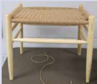
Chad Dawson Post & Rung Ash Stool Poly Finish & Woven Danish Paper Cord Seat
