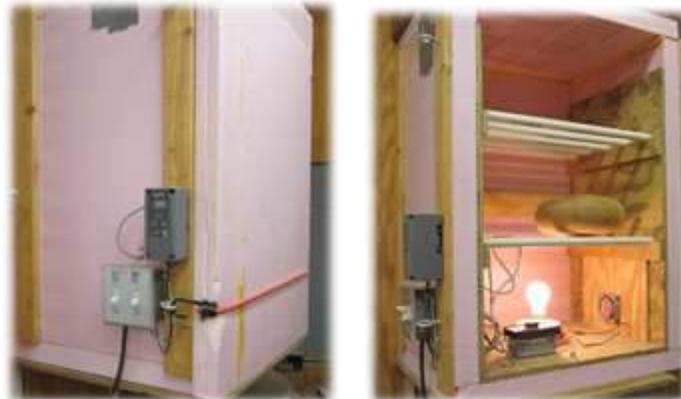
40 CFM axial fan controlled by a ceiling fan type speed control. A small 2" x 2" hole in the upper side opposite of
