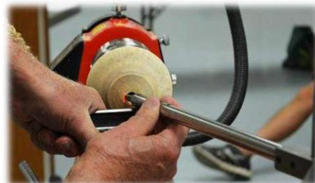
that is suspended outside the work piece to show the turner where their cutter is located inside the hollow
