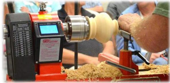
**Finishing** – Sanding of the exterior of the vessel could be done either before or after hollowing. Interior sanding should be limited to just the opening of the vessel. It is not necessary to try and sand the rest of the interior. After sanding apply your favorite finish.
