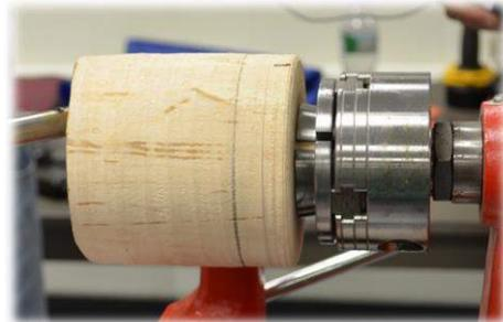
Mike shapes the outside of the vessel primarily using a 3/8 bowl gouge, using both a normal push cut as well as turning the gouge on its edge to shear scrape. Mike mentioned to be careful when turning the bottom of a cove because a gouge with high wings can catch on the opposite slope of the cove. To avoid this it is best to use a tool with swept back wings, such as a detail gouge.
