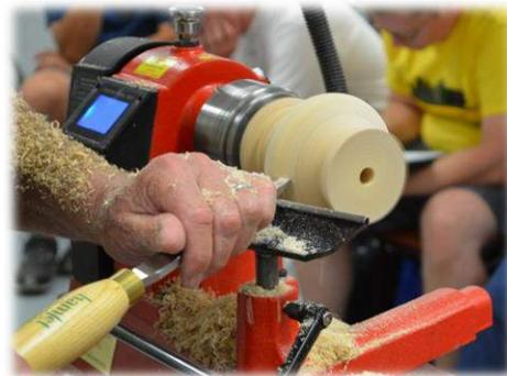
It was now time to hollow. Mike stated at this point he prefers to hollow dry wood as he has found that when working with green wood the shavings clog up in the vessel more than dry shavings do. Shavings in the vessel interfere with the scraper bevel making good contact with the wood. To overcome the challenge of not being able to see what is being cut while hollowing the Mini Monster Hollowing System (and other similar systems) has a laser
