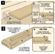
1. Using a straight bit in the router table, rout a stopped rabbet along the damaged edge. This will remove the chip-out and create a straight edge for accepting a filler strip.
