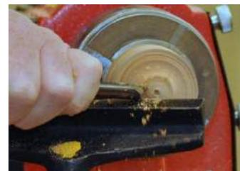
Inside of the body was final sanded. The top was pushed firmly into place and the top of the lid was finished with very light cuts so that the lid stayed in place with just the friction fit. Some edging at the joint between the lid and body was added for decoration. John noted that any final sanding and finishing work to the joined lid and body should be completed at this stage.
