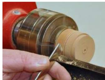
Moving on to the box bottom, John put the body bottom tenon into the chuck. He retested the lid's fit making sure it is slightly tight but not so tight as to crack the lid when pushed onto the body. The body was then hollowed out with either a rounded or squared inside design. John put a very slight chamfer on the edge of the central parting tenon so the lid would go on evenly and cleanly.
