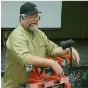
The woodturning tools John used in the demo and workshop were: 3/8" spindle gouge, 1/2" scraper, 1/8" parting tool, a 1/2" bedan, and a 1/2" skew. He first put the 2" by 2" by 6" piece of cherry hardwood between centers, turned it round, and added a 1/4" to 3/8" tenon on both ends. Each tenon was about 2" in diameter so they would fit securely into the #2 jaws on the chuck. He then secured one end of the wood into the chuck jaws using the tenon and supported the other end with the tail stock.
