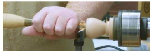
the standard lidded box. He warned that it requires more time when hollowing the body to make sure the hollowing depth and shape conforms with the outside body and base
