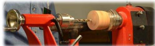
2. Drill a center hole through the end of the blank. This should be small enough that a finger will not fit through. This way nobody can test how well you have sanded the interior.
