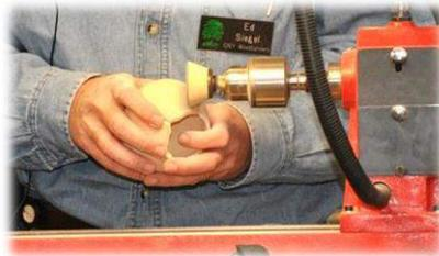
It is often joked that 60 or 80 grit paper is a shaping tool, here it is true. Hold the vessel in hand and press into the rotating sanding pad to shape. Sand between the petals, sand the lips of the petals, sand a line down the side wall
