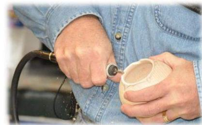
Do some light sanding then remove the piece from the lathe. For petal design an odd number of petals tends to look more natural than an even number. Draw out the
