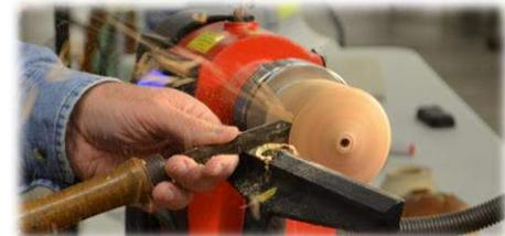
3. Turn the face of the insert slightly curved and sand.
