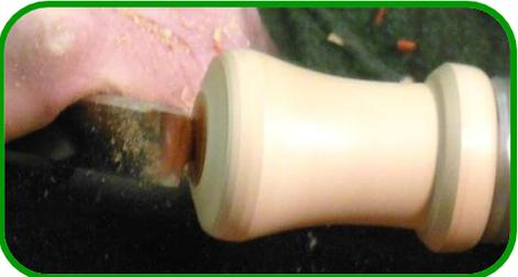
insert. Drill the hole. It doesn't have to be super deep but should at least match the length of your tenon. (If your tenon is too long, cut as needed.) Glue the piece in. Then turn your decorative wood to incorporate it into your stopper. If using stone or plastic cabochons measure the cabochon and turn an appropriate size area for the piece to be inserted. Make sure you make the recess deep enough. Glue the cabochon in then finish your stopper.
