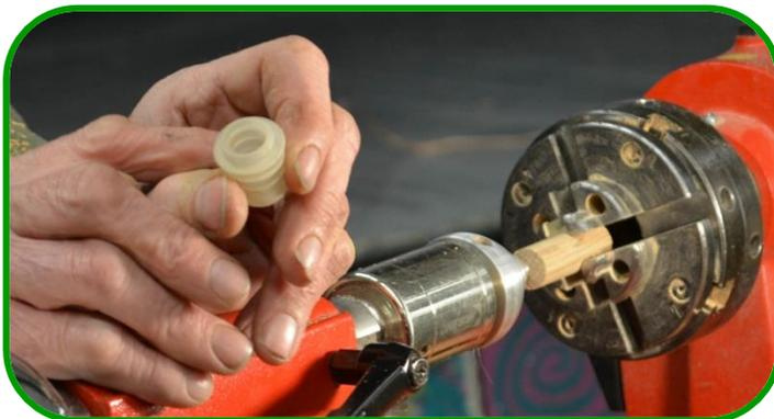
The next step was put the piece of dowel in a chuck and a tailstock and turn it down to fit inside the drilled stopper. That end of the dowel should be slightly shorter than the drilled depth and the dowel roughed up to hold glue. The dowel is then reversed in the chuck and tailstock and the other end turned down to 5/16" and of the correct length to hold the silicone stopper. The dowel is then glued into the stopper and allowed to dry.
