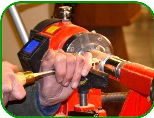
Don first turned the hardwood blank between centers so that it had a round tenon on one end. That tenon was used to hold the blank in a chuck while a 5/16" diameter hole was drilled in the other end ¾" deep using a drill chuck on the tailstock. After the drill chuck was removed, the tailstock was pulled up with a cone center put into the drilled hole. The drilled end of the blank was turned to the diameter wanted, finish sanded, and removed from the chuck.
