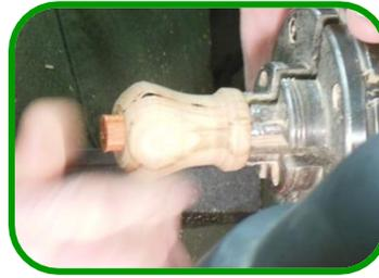
recess around it. Then measure your drill bit and turn a tenon on the contrasting wood piece to the size of the drill bit that will be used to create the recess for the wood
