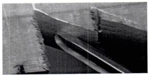
The final cut shape should be as shown in the photo, at this stage sand and finish, as it is difficult to do this in the final assembly.
