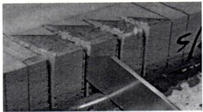
With a knife a cut into the edge at each end of the tree 8 cuts in all. This will insure that when removing the wood to form the tree, the wood does not split outside the tree profile, as these two faces are going to be glued together, if a split does occur this will give a gap in the joint.
