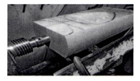
With a parting off tool, remove the areas between the double lines as shown, this allows access for the gouge when cutting the curved areas.
