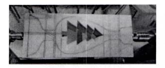
Next cut a Spigot on the base end to suit your chuck size, the maximum size will be 50mm diameter, as this is the size of the wood.
