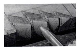
To get into the point of the tree profile, a finger gauge is necessary.
