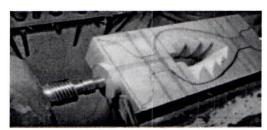
Remount the wood into the lathe using the chuck to hold the wood. Place the wood into the chuck with a loose fitting, engaged the tailstock with the hollow centre ensuring it fits original ring marks, and tighten the chuck up, this will ensure that the candlestick end runs true.
