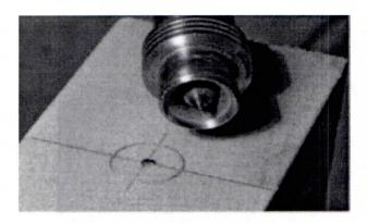
The use of the Hollow live centres at both the chuck and tailstock, this is important for safety, in the photo you can see the round circle which has been cut by the hollow centre in the wood end grain, this cut is into both pieces of wood, thereby clamping them within the centre, so as long as the pressure is maintained on the centres both pieces of wood are held fast by the hollow centres.
