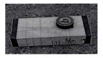
The wood assemble is now ready for turning, at each end mark the centre of the glue line, and make a small dimple hole.
