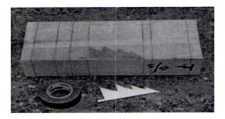
As you can see the two pieces of wood have been glued together with the outside faces marked o/s on the outside, and the T at the same end of each piece. It is important during the glueing operation to insure the faces are flat to each other.
