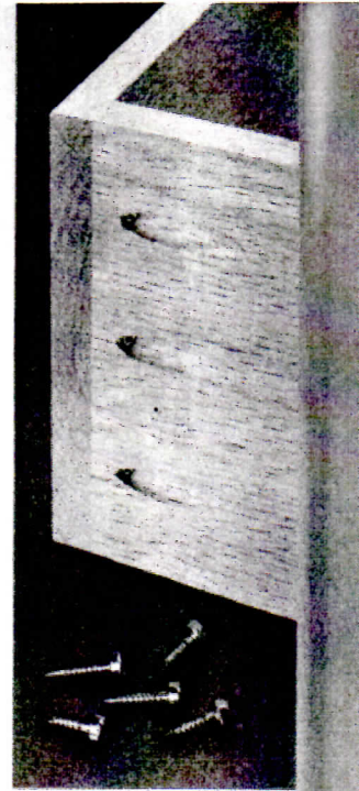
▲ Thin Stock. This box made of 1/2"-thick oak is an ideal use for panhead screws.
