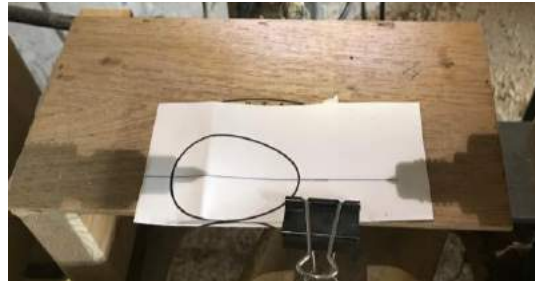
Align the template centerline with the shadows from the center points
