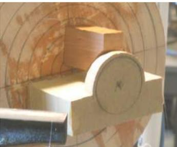
Ed attached double sided tape to the bottom of the piece and carefully centered the piece on the face plate using the center mark of
