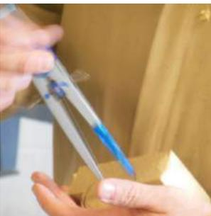
The next step in this challenge is to take one of the separated pieces and find the center of a bowl that can be made from the piece of hemisphere when turned 90 degrees to the original axis. Ed suggested using some simple
