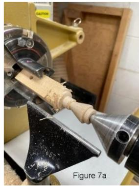
Prepare bottom of decoration to be slightly hollow. A steel screw can be inserted or a steel disk or random size steel piece glued to the underside of the decoration. Make sure materials are not stainless steel. If FHWS is used, drill pilot hole and countersink hole for flush FHWS insertion (**Figure 7**). Support the decoration with a cone tailstock unit and turn to desired shape, sand, finish, and then insert screw (**Figures 7a & 7b**).
