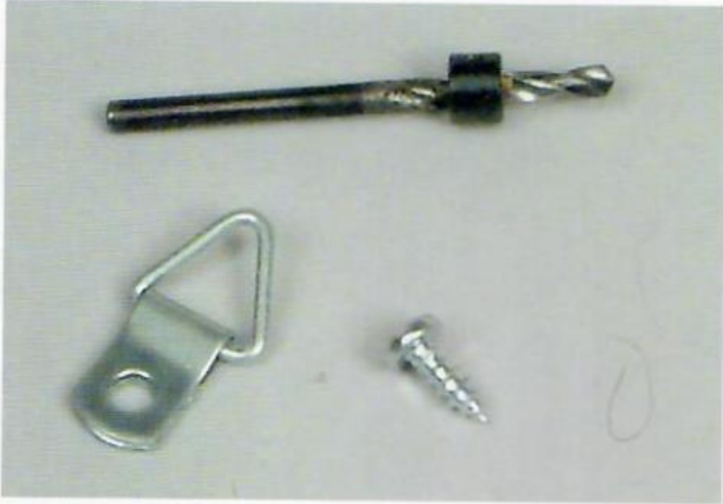
PHOTO 1.27 We use a mirror hanger instead of a saw tooth hanger because it is strong, reliable, and adjustable.
