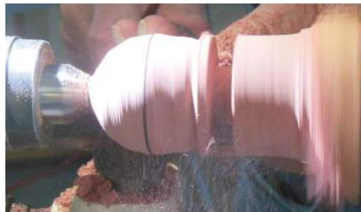
Then he used a parting tool to cut the end nearest the chuck to a depth that left
