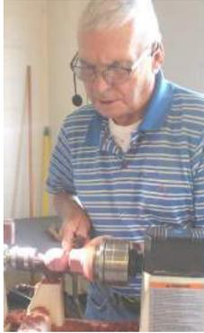
The hollowing process was done from the open end of the piece through the 1/2" drill hole using a small angled hollowing tool. Dick talked about small hollowing tools (angled scraper) that could be purchased on line or those that could be made at home. He explained that hollowing should leave about 1/8" to 1/4"
