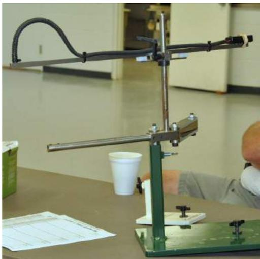
indicator that pointed where the hollowing tip was inside the body. Dick explained that not using a jig could be compensated for by marking the depth desired on the shaft of the tool and learning to feel where it was cutting inside sight unseen.
