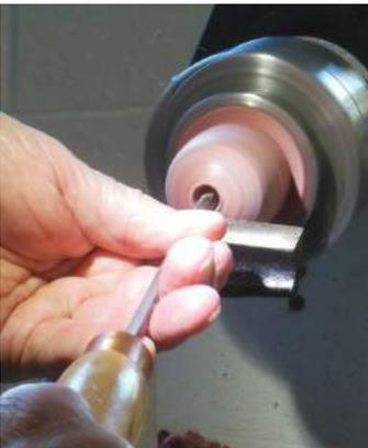
in the walls and with the inside as smooth as possible. Start hollowing just inside the 1/2" entrance hole by scrapping to the left and then taking off layers inside by starting at the
