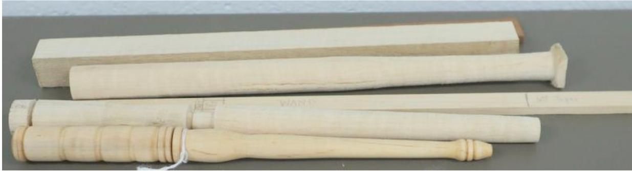
Blank size is 1-inch square x 13-5/8" long – that is the throat of my bandsaw. Mark centers on both ends of blank, dimple with awl. Mount blank between centers and use a roughing gouge to turn it round. I will usually put a rough taper on the round blank.
