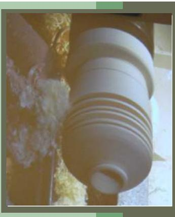
and of uniform thickness. The slot was the width of the parting tool that was kept very sharp from repeated use of the grinder or a hand held diamond hone. Ed kept the speed up around 1,500 rpm's to get a clean cut.
