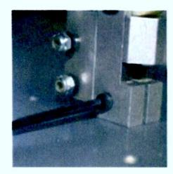
To help prevent setscrew from moving off center, a dab of blue loctite, paint or nail polish works very well. Do not use red loctite as it will cause the screw to bond in place making it very difficult to remove
