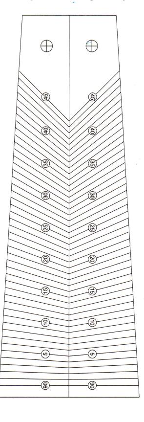
Tired of bending over and trying to read the table tilt gauge on your scroll saw or band saw? Use this handy table tilt gauge on top of your scroll saw or band saw table instead! When completed as instructed below it can be used to set a table tilted to the left or right.
