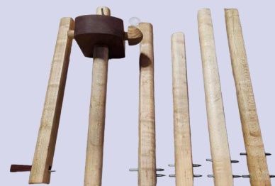
Jeff Handel Marking Gauge Mahogany, Birdseye Maple, & Bloodwood w/Homemade Paste Wax Made with Only Hand Tools
